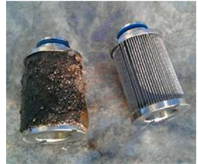
Filter clogging due to bacteria and particulate deposition
