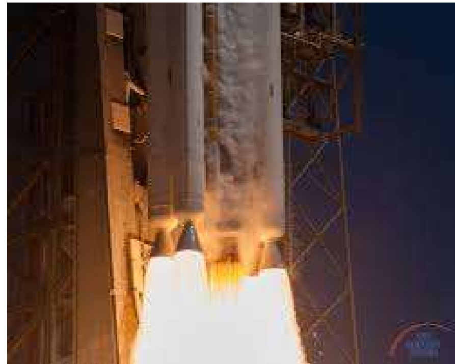
Atlas V 541 lift-off: RD-180 and four solid motors AJ-60A
