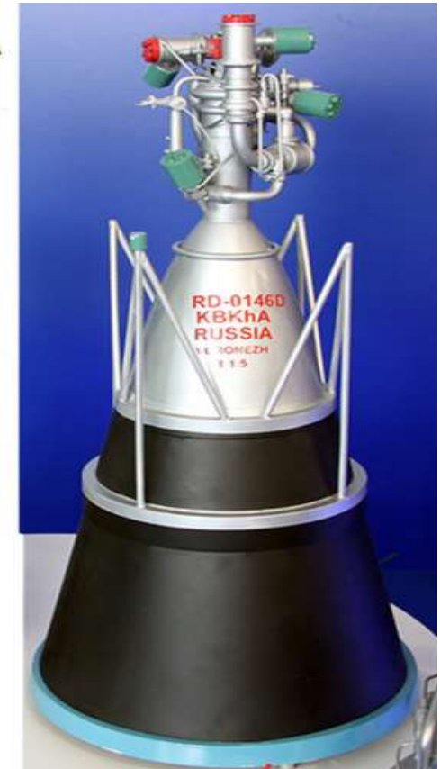
RD-0146 supposed to fly on Angara 5, LOX/LH 2 expander cycle engine
