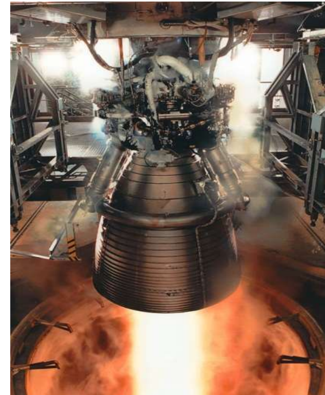
Vulcain 2: Cryogenic (LOX/LH 2 ) Gas Generator Engine
