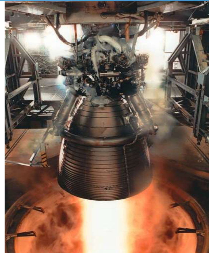
Vulcain 2 engine of Ariane 5, cryogenic (LOX/LH 2 ); Gas Generator Cycle
